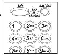
If the **TALK/BATT LOW** LED begins to flash, the phone is programmed to eliminate its functions to save power. The table below describes what to do to return your phone to normal operation.
